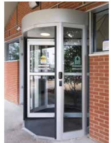
Because there is no curved glass, segmented drums have easier installation and lower costs than round drums and allow for immediate glass replacement when needed.
